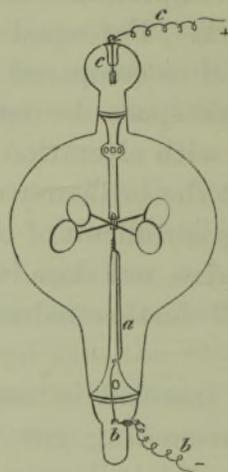
through the glass. The other terminal, *c*, passes through the top of the bulb, and is of aluminium wire inside. The vanes are of aluminium, lampblacked on one side, and connected by aluminium arms to a hard steel cup; the whole fly is therefore in metallic connection with the lower terminal.
