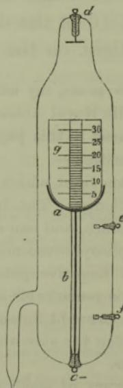
cylinder, 22 millims. diameter, accurately made of polished aluminium; it is supported in position by the glass tube *b*, through which passes a fine copper wire connecting
