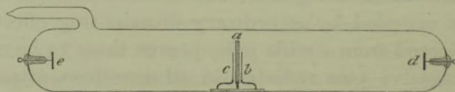
manner:—In the centre of a tube, furnished with flat aluminium terminals, *d*, *e*, is supported a plate of uranium glass, *a*. About half a millimetre on one side is a film of uranium glass, *b*, and on the other side a similar film of German glass, *c*. The two films are thin enough to show brilliant colours of thin plates when viewed by
