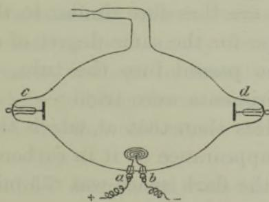
in contact, and the ends are sealed in separately, so that the spiral can be made red hot by connecting the wires *a* and *b* with a battery. *c* and *d* are two flat aluminium poles. An apparatus was connected with the pump whereby different gases could be introduced into the bulb and experimented with at different pressures.
